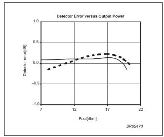
Figure 12. Detector error vs. output power
